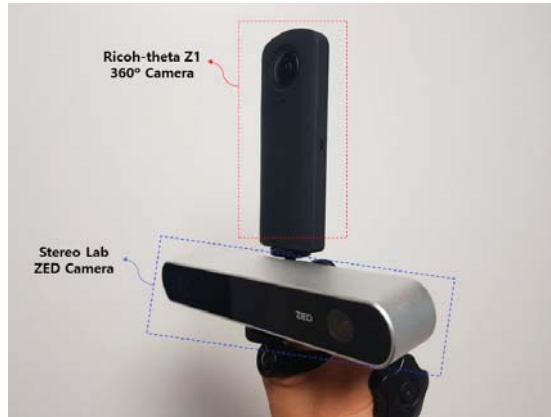
Figure 4. 360° camera and stereo-vision ZED camera.
