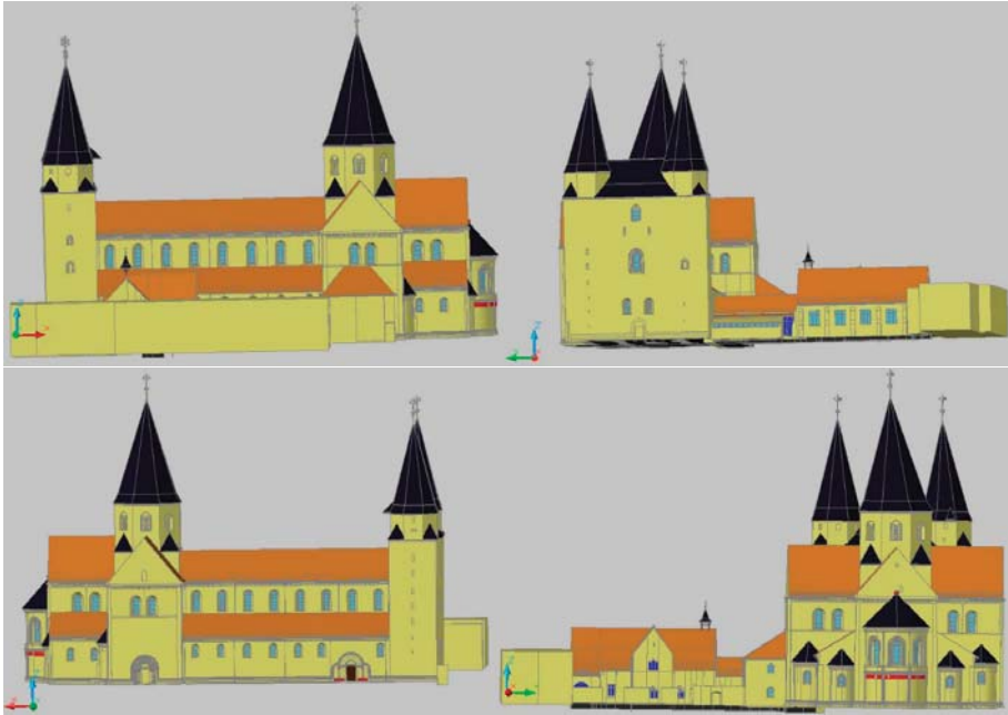
Figure 4. Constructed 3D model of the imperial cathedral in Königslutter, Germany—View of the four fronts in AutoCAD.
