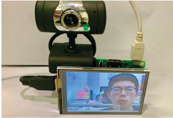
Figure 8. Physical photo of Lip Reading System on Raspberry Pi.
