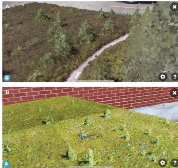
Figure 13. Videos illustrating a screen recording of the AR visualization of the (A) SfM and (B) LiDAR point clouds through the iOS Sketchfab application. The models can be viewed in AR at https://skfb.ly/onuU9 (LiDAR) (accessed on 14 April 2021) and https://skfb.ly/onuUs (SfM) (accessed on 14 April 2021).
