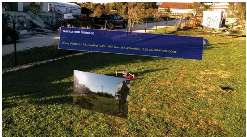
Figure 3. The AR Ego-centric View mode. The AR user can be shown in collinearity between the user and the drone's camera in the right corner.
