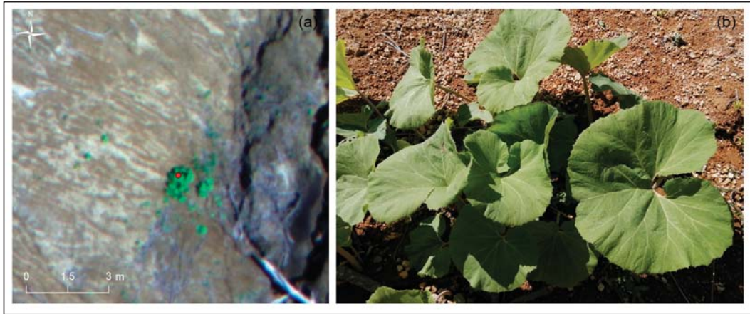
Figure 3. (a) The red dot is the vegetation class obtained by ODK with the RTK system accuracy (2 cm) on the Multispectral UAV ortho-mosaic in true color, and (b) the respective photo of a Japanese sweet-coltfoot for verification on 12 May.
