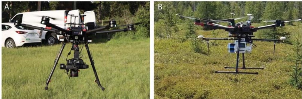
Figure 2. M600P RTK enabled UAV with the (A) Canon DSLR and (B) LiAIR S220.
