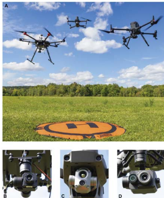
Figure 1. RPAS systems and cameras in this study. (A) The M600P (left), M2EA (center) and M300 (right). (B) the Zenmuse XT-R with gimbal, (C) the M2EA form-integrated thermal (upper) and visible (lower) cameras and, (D) the Zenmuse XT2 thermal (right) and visible (left) cameras. The cameras are shown in the same order from L-R as the airframes with which they are compatible.
