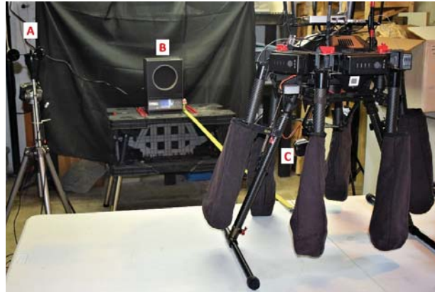
Figure 3. Validation set-up that would be typical of a workspace pre/post RPAS operations. The tripod (A) that carries the environmental sensors for air temperature, RH, pressure and air movement, the FLUKE 4180 blackbody (B) and the M600P airframe with the XT-R camera (C).
