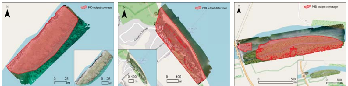
Figure 5. AgiSoft vs. P4D with Dataset B (left), Dataset C (middle), and Dataset E (right). The red shade and the inset at the bottom right corner are the coverage of the orthomosaic generated by P4D. The red cluster scattered in the shade is voids that have no value in the orthomosaic datasets. This is overlaid with the output from AgiSoft to show the difference of coverage.
