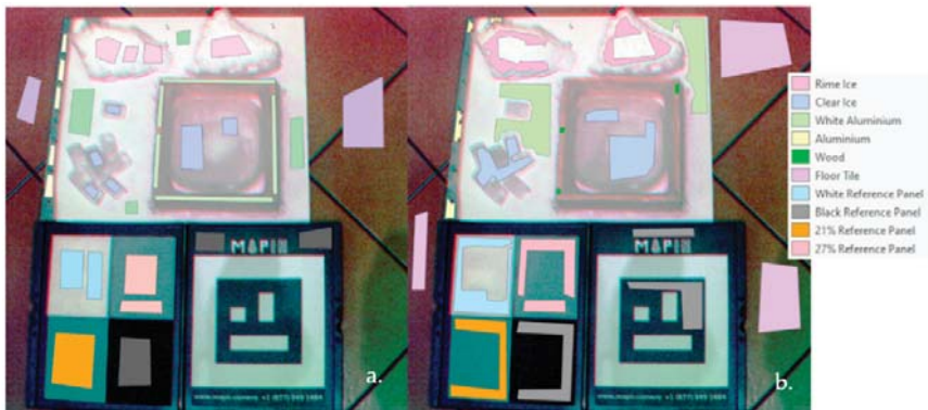
Figure 3. Example of annotated image with reference data. Training set sample (a) and validation set sample (b).
