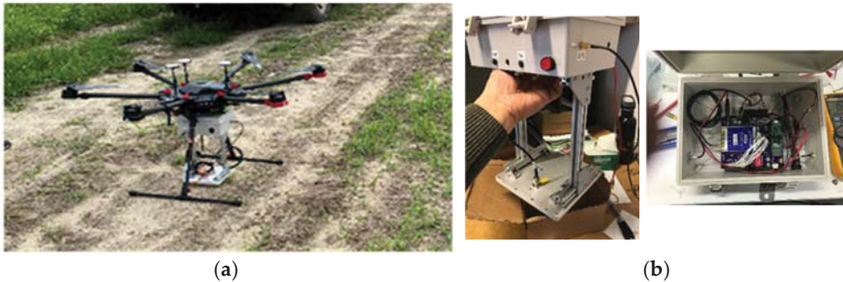
Figure 1. (a) DJI Matrice 600 Pro, and (b) RFID Reader Module (RFID-RM).
