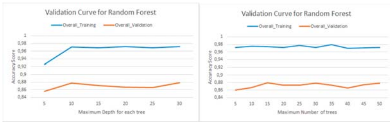
Figure 8. RF validation curve for maximum depth (on the left) and maximum number of trees (on the right).
