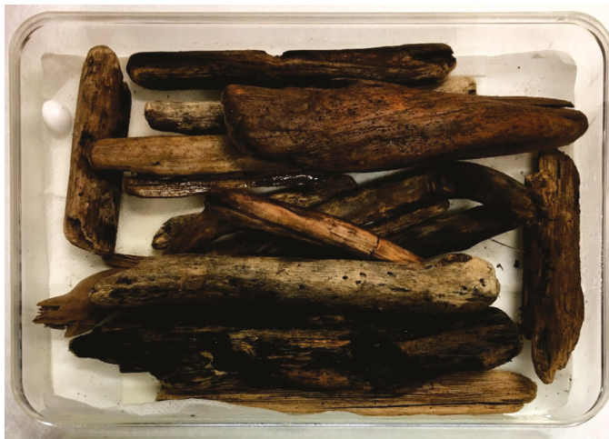
Figure 7. Example of a driftwood damp chamber; note the use of a camphor ball for the prevention of mites.
