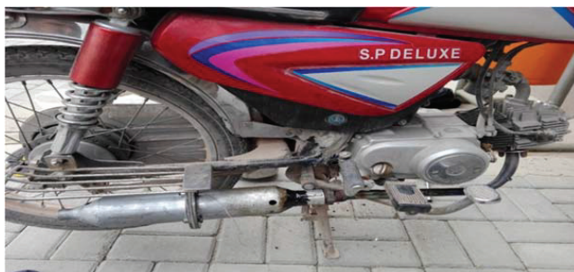
Figure 17. Catalytic converter mounted on engine exhaust for testing
