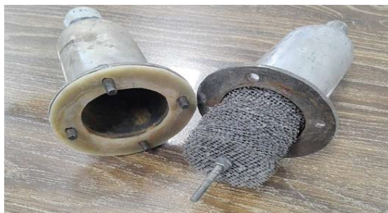
Figure 16. Coated wire meshes arrangement
