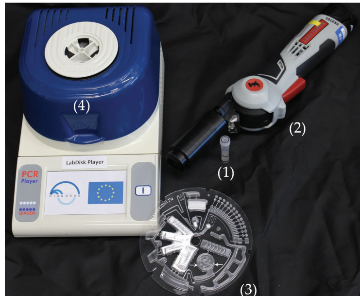
Figure 3. Image of the items which comprise the experimental setup. (1) Tube containing the mixture of the saliva sample, S. marinus control bacterium and steel beads. (2) Hand-held device (Terralyzer), into which the tube is inserted for performing the mechanical lysis and saliva homogenization. (3) The OralDisk, where the lysate is pipetted in the chamber indicated by the two white arrows. (4) The LabDisk Player instrument that performs the OralDisk processing and real-time PCR.
