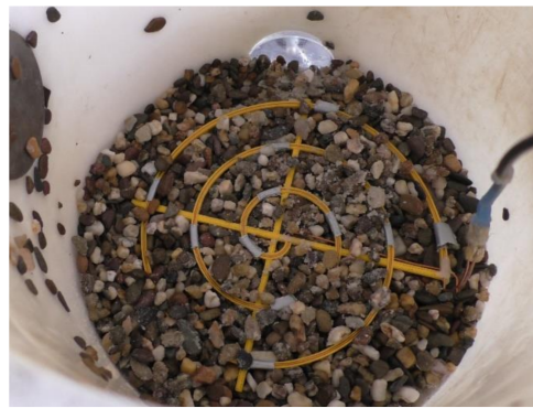
Figure 7. Flat coil sensor embedded in the proctor mould.
