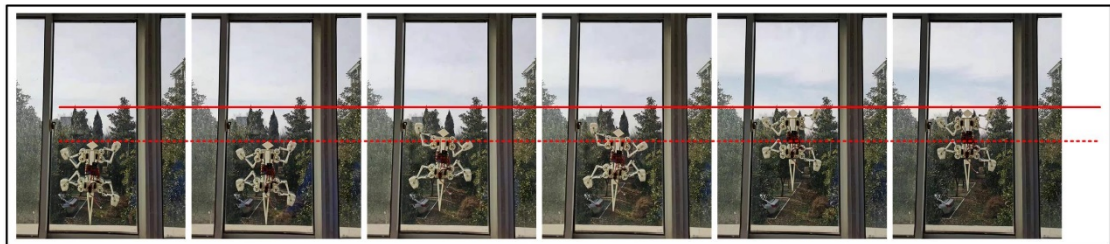
Figure 13. Experiment of the locomotion of the bionic robot climbing on the glass surface in cycle.
