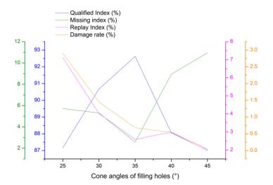
Figure 10. The relation curve between cone angles of filling hole and seed performance.
