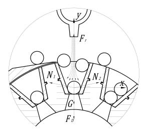
Figure 4. The force map of the seed pressed to the bottom of the hole.
