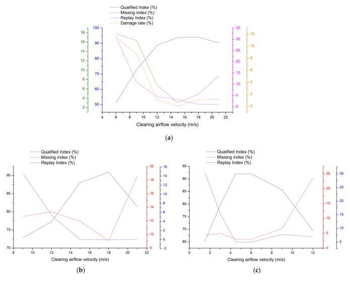
Figure 7. The relation curve between seed cleaning airflow velocity and seed performance (a) Soybean; (b) Corn; (c) Rape.
