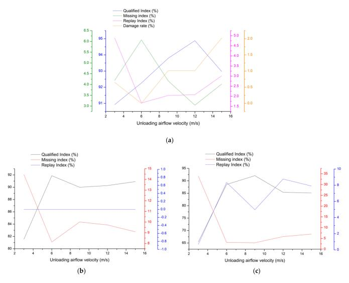
Figure 8. The relation curve between seed unloading airflow velocity and seed performance (a) Soybean; (b) Corn; (c) Rape.
