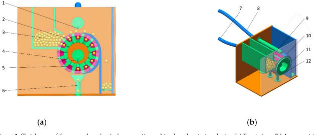
**Figure 1.** Sketch map of the general mechanical pneumatic combined seed metering device. (**a**) Front view; (**b**) Axonometric view. 1. Seed cleaning nozzle; 2. Seed filling hole; 3. Seed filling box; 4. Seed unloading nozzle; 5. Unloading seed pore; 6. Seed cup; 7. Seed unloading duct; 8. Seed cleaning duct; 9. Seed strips; 10. Protective seed plate; 11. Seed collection box; 12. Feeding drum.
