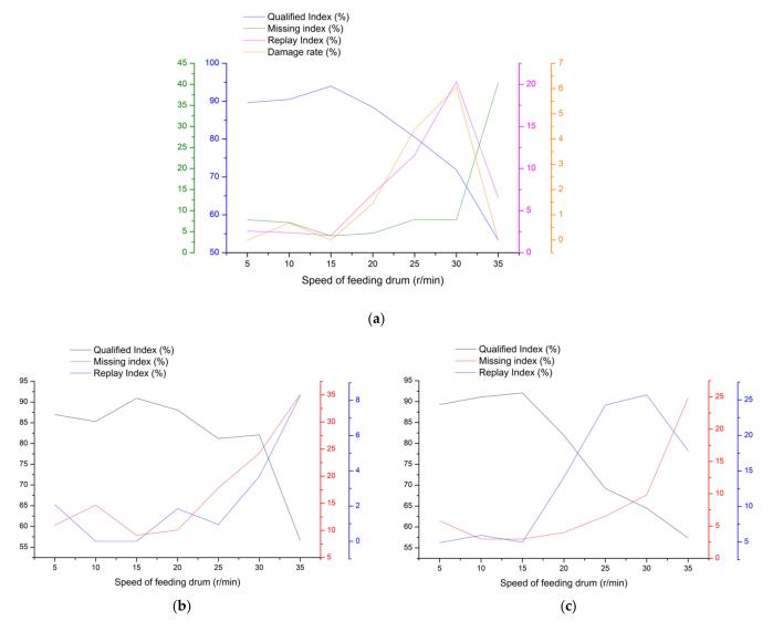
Figure 9. The relation curve between speed of the feeding drum and seed performance (a) Soybean; (b) Corn; (c) Rape.
