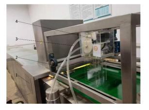
**Figure 6.** Indoor seeding test. 1. JPS-12 seeding performance test bed; 2. Seed unloading duct; 3. Seed cleaning duct; 4. Seed metering.
