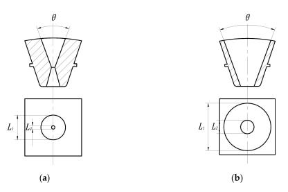
Figure 2. Sketch map of seed filling holes. (a) Small seed filling hole; (b) Big seed filling hole.
