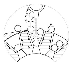
Figure 5. The force map of seeds cleaned out of filling hole.
