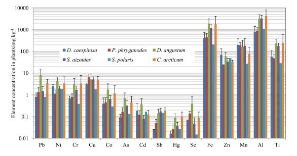
**Figure 2.** Element concentration means in the six species of plants, with error bars of one standard deviation. The sample numbers of plants *D. caespitosa*, *P. phryganodes*, *D. angustum*, *S. aizoides*, *S. Polaris*, and *C. arcticum* are 2, 3, 6, 4, 1, and 3, respectively. Note that a base-10 log scale is used for the *y*-axis of element concentrations.
