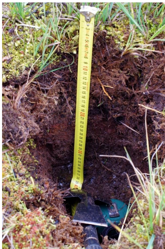
Figure 11. The features of soil profile (section) at the heaving (frozen) peat mound in the Adyr-Khem river valley (Volkova, 2021).
