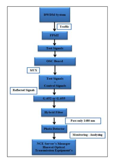
fiber burns, fiber contamination, etc., are reflected back to the transmitter side and filtered from the traffic signal by the FPMT technique and then analyzed to confirm the root cause.
