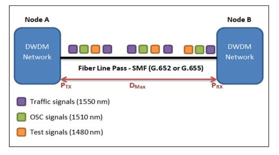
**Figure 7.** All the signal flows over the fiber line and the maximum distance to transmit the signal between two nodes.
