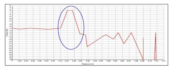
**Figure 11.** Event is Fiber break (standard SMF G.655 at 1550 nm was used and FPMT test signal was transmitted by the OSC board).
