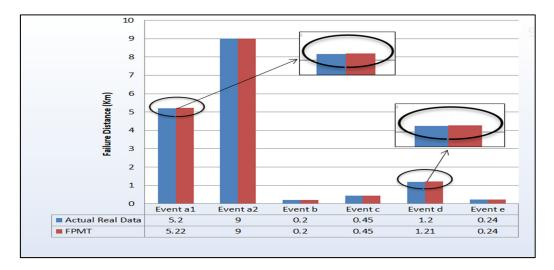
Figure 15. Real fault locations and fault locations detected by FPMT.
