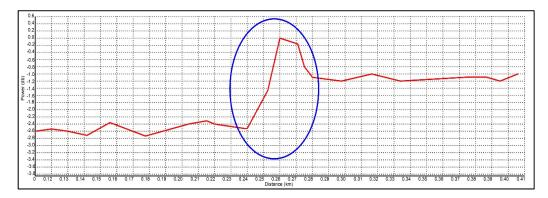
**Figure 13.** The fiber interconnection event between fiber cables G652 and G653 and the FPMT test signals transmitted by the OSC board.
