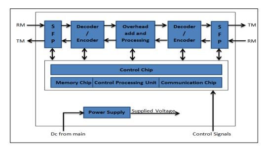
4.1. The OSC Board before and after Integrating the Implemented FPMT Technique Detection Circuit
