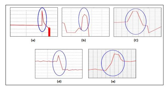
Figure 14. Pattern of the reflected test signals during fiber line detection.
