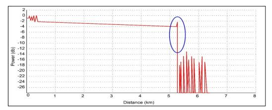
**Figure 8.** Fiber break event (standard SMF G.652 at 1550 nm used and FPMT test signal was transmitted by the OSC board).
