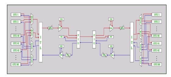
**Figure 1.** The ultra-high speed data transmission optical system structure by implementing an 80-channel DWDM system.
