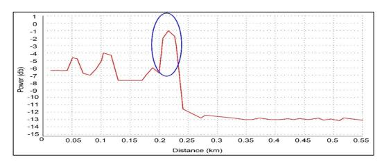
**Figure 10.** Event is Fiber end face contamination (standard SMF G.652 at 1550 nm was used and FPMT test signal was transmitted by the OSC board).
