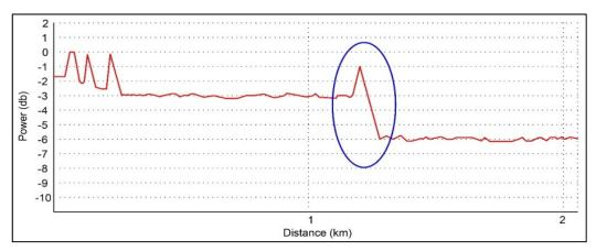
**Figure 12.** Event is fiber large insertion loss on the connector the (standard SMF G.652 at 1550 nm was used and FPMT test signal was transmitted by the OSC board).
