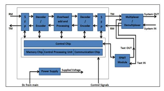
Figure 6. The OSC board block diagram after integrating the FPMT detection circuit.
