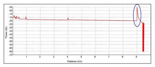
**Figure 9.** Fiber break event (standard SMF G.655 at 1550 nm was used and FPMT test signal was transmitted by the OSC board).
