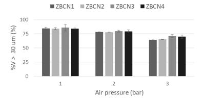
**Figure 7.** Dependence between the air pressure and the volumetric share of the droplets with diameters greater than  $30 \,\mu\text{m}$ .
