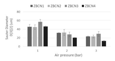
Figure 5. Dependence between the volume-surface diameter and air pressure.
