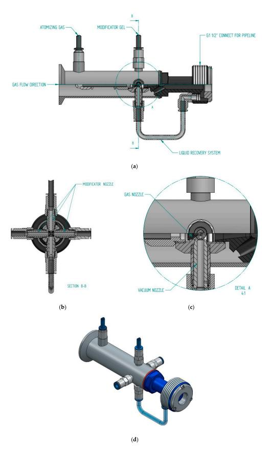
**Figure 2.** The catalyst atomizing nozzle: (**a**) construction, (**b**) B-B section, (**c**) the position of the liquid nozzle, (**d**) visualization.
