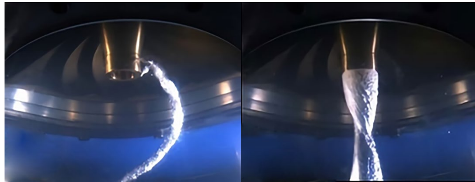
Figure 5. Vortex rope structure [20].
