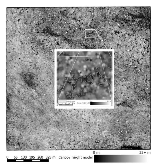
**Figure 2.** Example (landscape no. 89, see Figure 1a for its exact position in the southeast of the study area) of a canopy height model derived from aerial LiDAR data used to detect forest gaps (hatched zones in the insert) (gap height threshold = 5 m).
