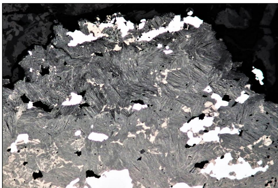
Figure 16. Eskebornite (light-brown) and clausthalite (bright) largely replaced by unknown Cu–Fe selenites (light-grey to dark-grey) of strongly varying Cu/Fe ratios, from Cu > Fe to Cu = Fe to Cu < Fe, possibly representing chalcomenite and mandarinoite. The darker the domains are, the more Fe-rich is the alteration mineral. Reflected light image, 500- \mu\text{m} -wide, plane polarized light.
