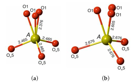
**Figure 5.** Coordination of the *A* site in natural (**a**) and synthetic (**b**) natrophosphate at room temperature. Legend as in Figure 4. The interatomic distances are given in Å.
