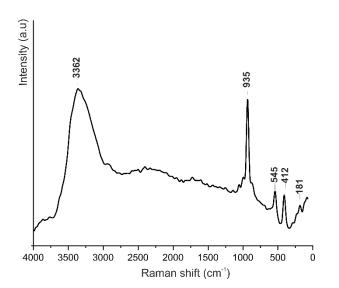
Figure 3. Raman spectrum of natural natrophosphate.
