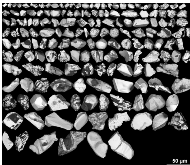
Figure 2. A mosaic of 166 precious metals minerals (PMM) excluding Au is automatically generated by the routine. These PMM include various species of platinum-group elements-bearing and Ag-bearing minerals found in till samples collected in the Nunavik area (Quebec, Canada).
