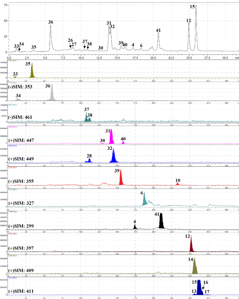
Figure 4. HPLC-DAD chromatogram (330 nm; (a) and some HPLC-ESI-MS chromatograms (SIM mode, positive/negative ionization; (b) of methanol extract of P. sibiricus herb. Compounds are numbered as listed in Table 2.
