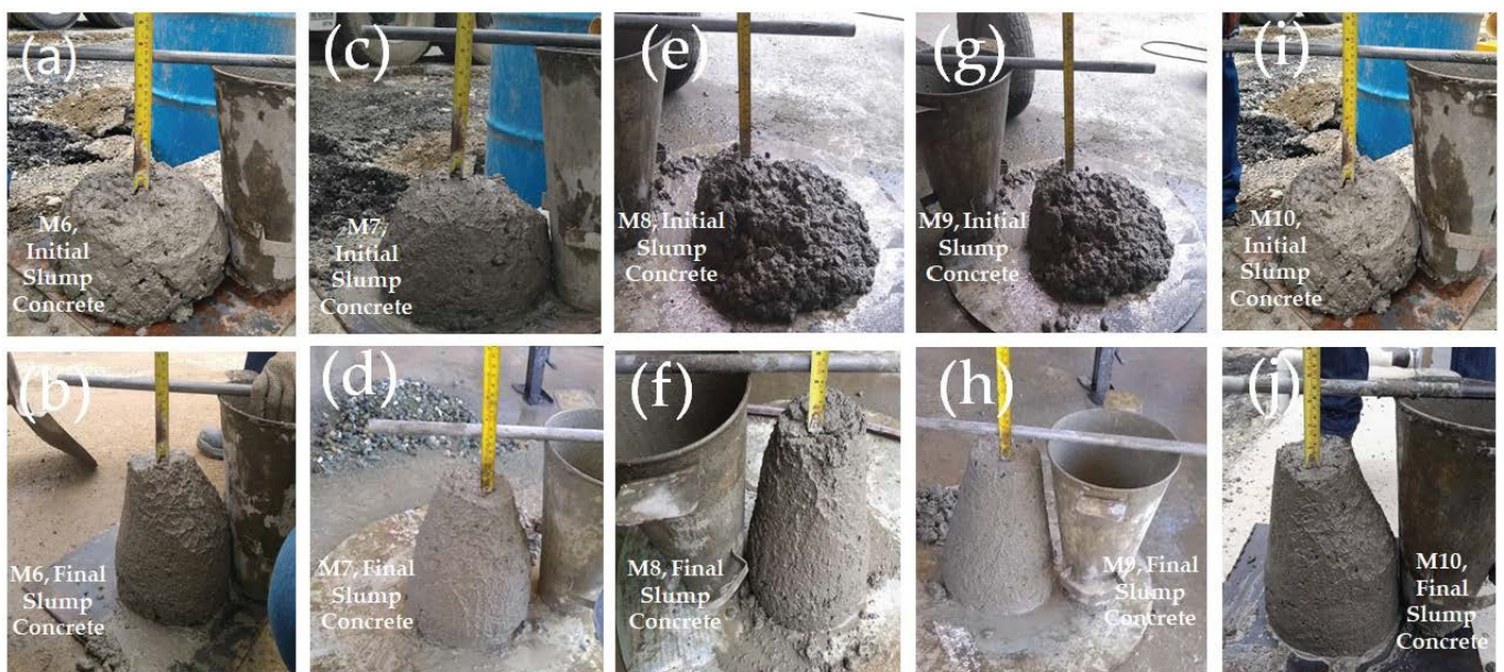
Figure 9. Standard ASTM C143 of the five mixtures evaluated with metakaolin, showing the initial and final slumps.
