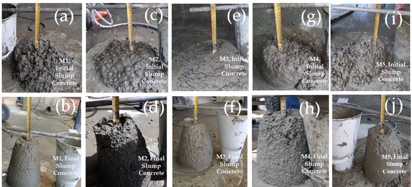
Figure 7. Figure of the slump, standard ASTM C143 of the five mixtures evaluated with residual aggregate powder, shows the initial and final slumps.
