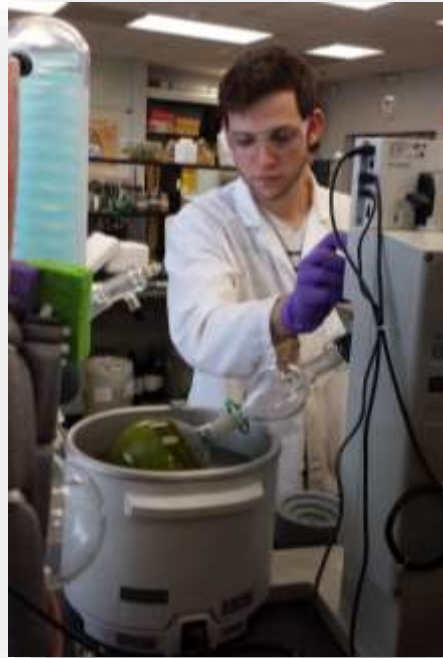
Solvent removed under reduced pressure with a rotary evaporator
