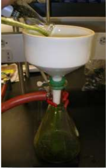
Plant materials separated from extract with vacuum filtration
