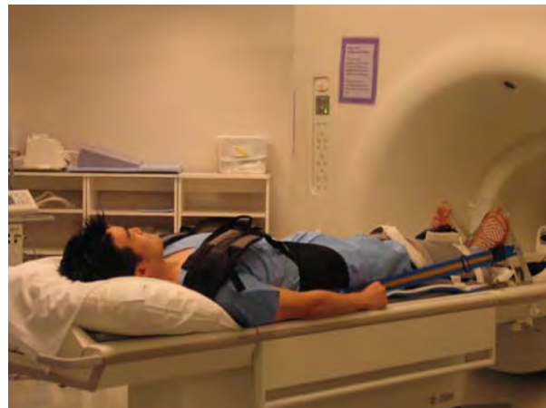
Figure 1. A subject is ready to be scanned at the 1.5T by Gilwoo Choi, MS (collaboration of Radiology, Mechanical Engineering and Vascular Surgery). The study includes imaging of the femoral arteries with a new MR-safe device that simulates weightbearing on a subjects lying in the supine position (B. Krasnow, Mag Design & Engineering, MagConcept.com).
