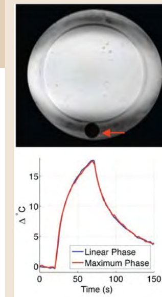
Left: Image of the phantom acquired before heating, using the proposed pulse design. The red arrow indicates an oil-filled vial, confirming fat suppression. The hot spot was in the phantom's center. Right: Temperature measured in the voxel corresponding to the hot spot center indicated in Fig. 1. Excellent agreement is observed between maps acquired with the two pulses.
