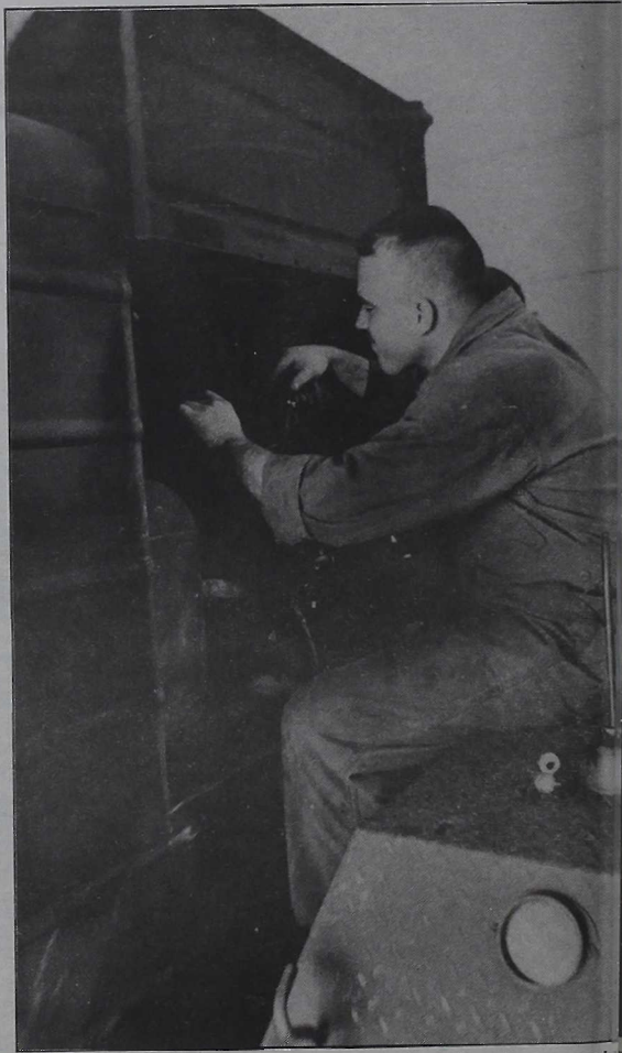
Above, motor transport Marine, LCpl. Anthony Leach, a reservist from Tampa, Fla., repairs a high pressure lube unit in the RBE Co. Below, motor transport section. Left, 50 percent of the company's responsibility is paperwork. GySgt. Walter Coleman, HQ Btry., 10th Marine works in the RBE Co. filling out equipment repair orders.
