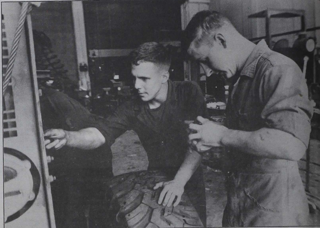
Engineers, Cpl. Russell Kelso, 2nd CEB and LCpl. David Anderson, a reservist assigned to 2nd CEB, repair a forklift's hydraulic filter.
