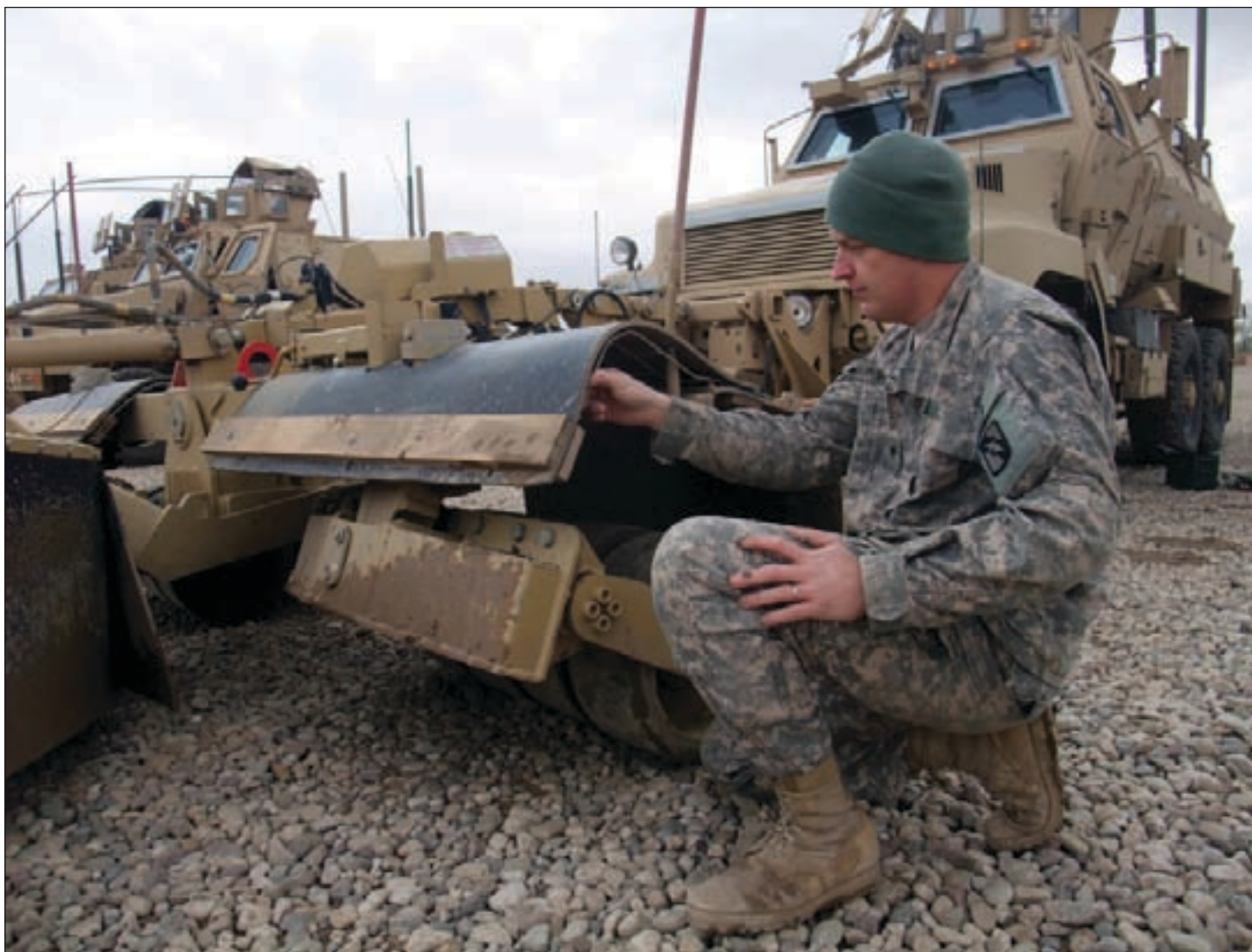
Spc. Michael A. Boucher, a gun truck driver and a Batesville, Miss., native, explains how he made additional mud flaps for the Self-Protection Adaptive Roller Kit, which absorbs bomb damage and shields the vehicle and crew, in his company motor pool Feb. 4 at Contingency Operating Base Q-West, Iraq. Boucher serves with 1st Platoon, B Company, 2nd Battalion, 198th Combined Arms, 155th Heavy Brigade Combat Team out of Greenwood, Miss., 13th Sustainment Command (Expeditionary).
