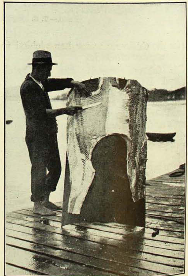
Cutting attached flesh from the shark's hide on a beam- ing board. The right half still has pieces of flesh attached to it; the left half has been carefully cleaned. [Photo.—T. C. Roughley]
