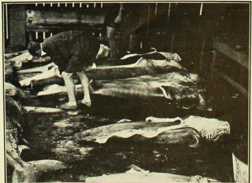
After the removal of the fins, the skin is cut down the back and behind the gills, preparatory to stripping.
