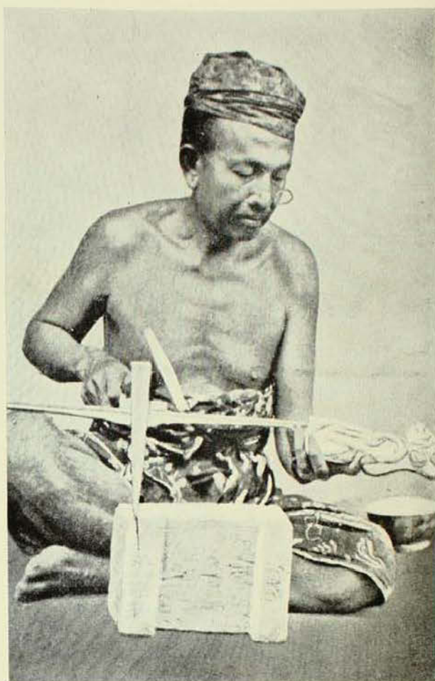
A Balinese silversmith using a hammer and punch to emboss a design on a bowl. He is wearing batik skirts on which elaborate patterns are printed by a complicated wax and dyeing process.
