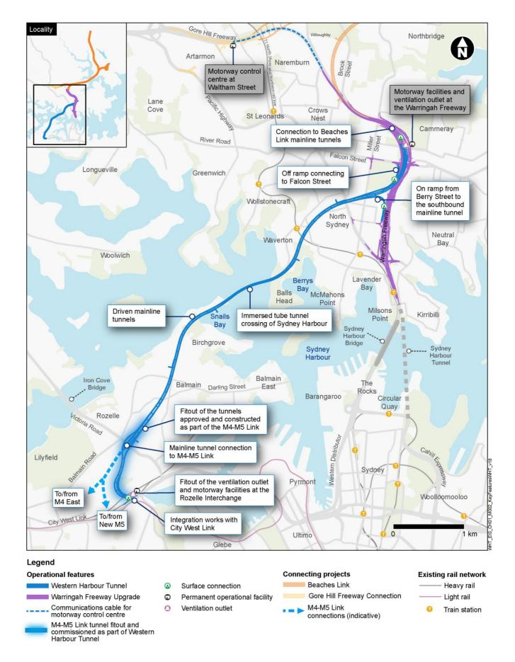
Figure 1-1 Key features of the Western Harbour Tunnel component of the project
