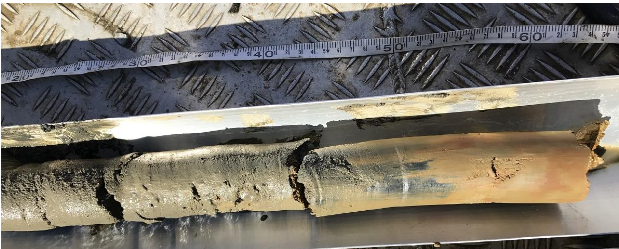
Photo 2 Grey brown silty sand with shell overlying stiff orange brown clay observed at Birchgrove end of the dredge area (core WHT5)
