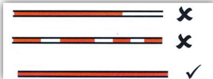
Figure 6: Correct Filling of the Capillary Tube (Used with permission, Radiometer 2008b)
