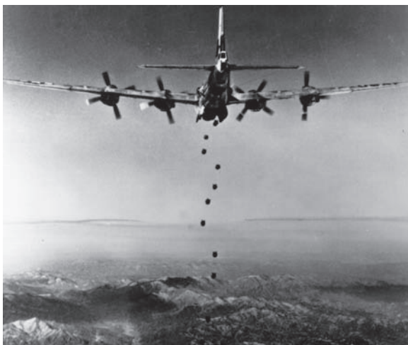
Figure 10. The B-29 carried the 12,000 pound TARZON (VB), used during the Korean War.
