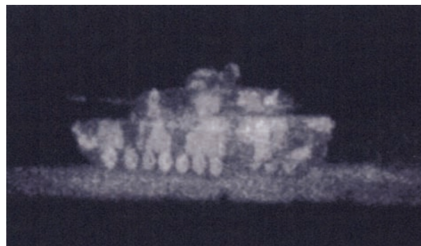
Figure 6. Example of laser-illuminated imagery. Note that because the laser sends out the light in pulses, only the region about the object is illuminated. This allows the camera to ignore scattered returns from intervening obscurants such as smoke and dust.
