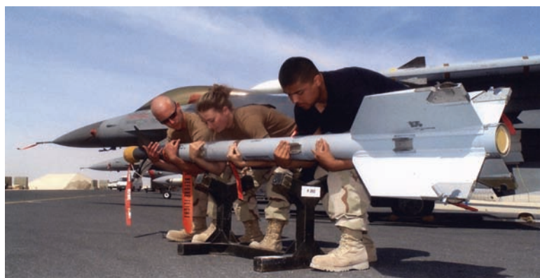
Figure 9. From left, Airman 1st Class Bradley Smith, Staff Sergeant Jessica German and Airman 1st Class Gerardo Gonzalez hoist an AIM-9 Sidewinder missile before mounting it to an F-16 Fighting Falcon aircraft. The airmen are assigned to the 379th Expeditionary Aircraft Maintenance Squadron at a forward-deployed location in Southwest Asia supporting Operation Enduring Freedom. (Photo by Master Sergeant Terry L. Blevins)
