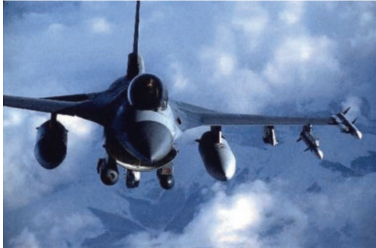
Figure 4. LANTIRN – An F-16C/D Fighting Falcon fighter plane with LANTIRN pods mounted externally beneath the body of the aircraft. On the left, the targeting pod; on the right, the navigation pod.
