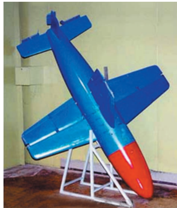
Figure 8. The VB-9 guided bomb, equipped with a radar seeker.
