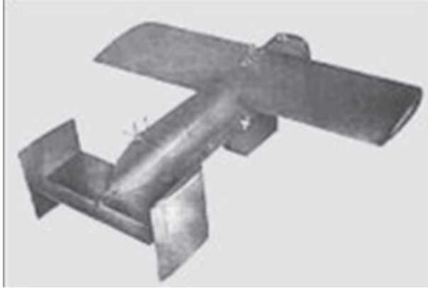
Figure 7. The GB-4 (above) was a GB-1 (AZON) with an added television camera and radio remote control, which during testing achieved an impressive 200 foot CEP.
