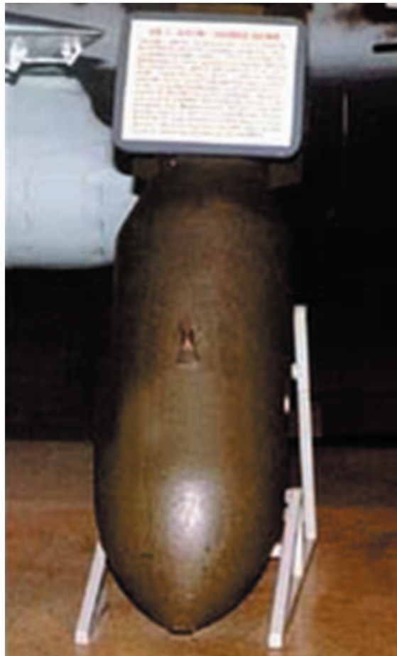
Figure 8. The VB or vertical bomb series, (below) consisting of 1,000 pound bombs fitted with a steerable tail assembly and a tracking flare that were ultimately equipped with a radio control system, allowing a bombardier to direct the bomb to a target using a joystick.
