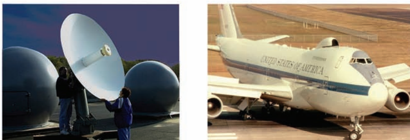
Figure 5. Shipboard and Airborne Terminals —WSC-6 shipboard (left) and ASC-24 airborne on the E4B aircraft (right).
