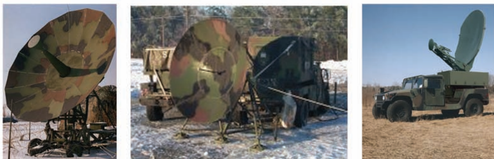
Figure 4. Transport Terminals - 20 foot AN/TSC-85 (left), 8 foot AN/TSC-93 (middle), and 2.4 meter triband (right).
