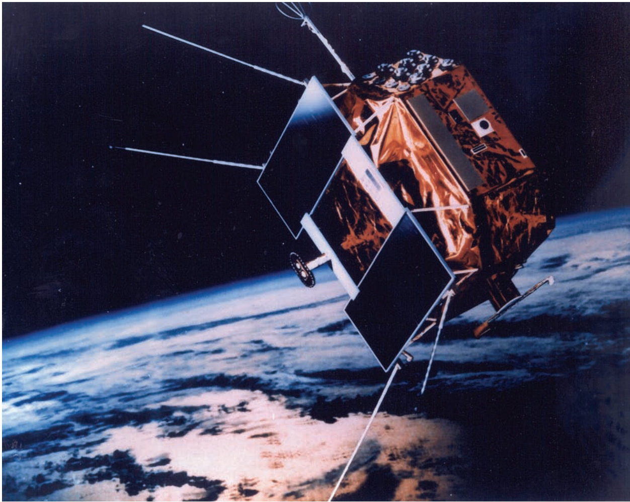
The Combined Release/Radiation Effects Satellite was configured for a rocket-launched, single-orbit mission in 1987. Its solar panels have been drawn in to fit them to the fairing for the rocket.
