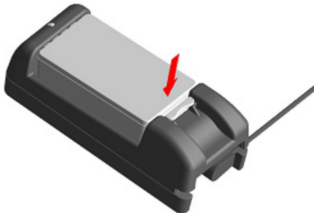
Figure 17-6 Battery Pack Installation (2)
