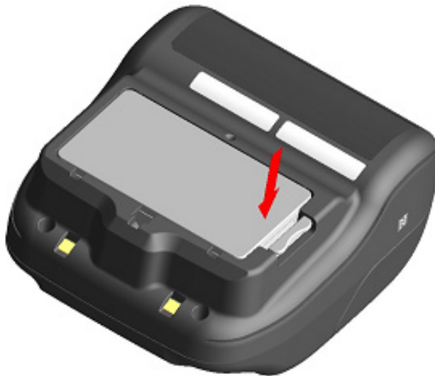
Figure 8-3 Installing Battery Pack (2)
