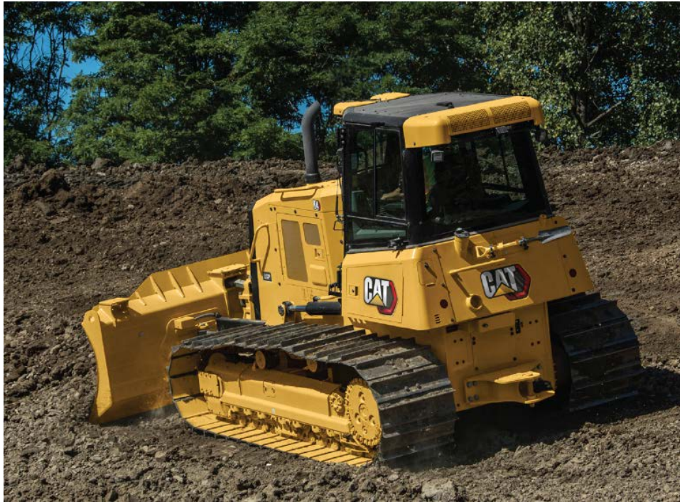
Description: D4 Dozer
