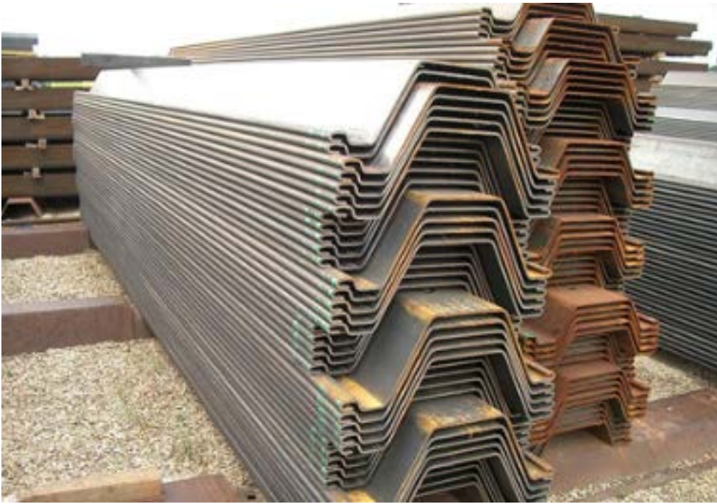
Description: Sheet piles are long structural sections of steel with interlocking edges that are driven into the ground to create a continuous wall.
