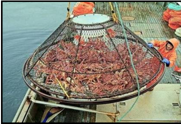
Conical crab pot Dimensions: 88" base diameter x 32" tall, 27.5" top opening
