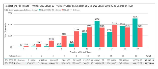
Figure 17 - Side-by-side comparison of SQL Server 2008 R2 with 16 vCores vs SQL Server 2017 with 4 vCores
