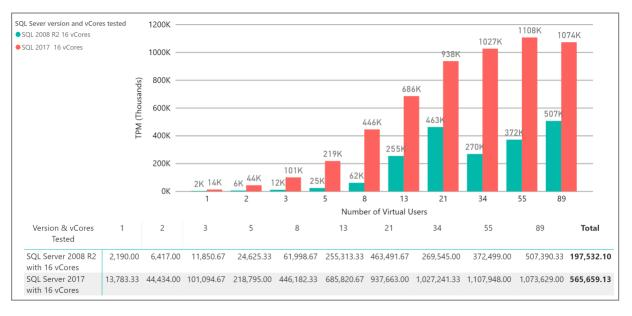
Figure 13 - Comparing SQL Server 2008 R2 on HDD vs SQL Server 2017 with DC500M drives with 16 vCores
