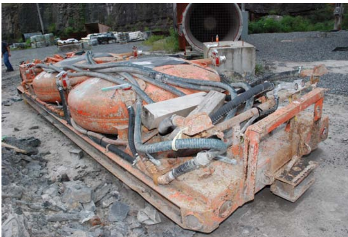
UBB’s orange pod duster, above, and white rock duster, below
