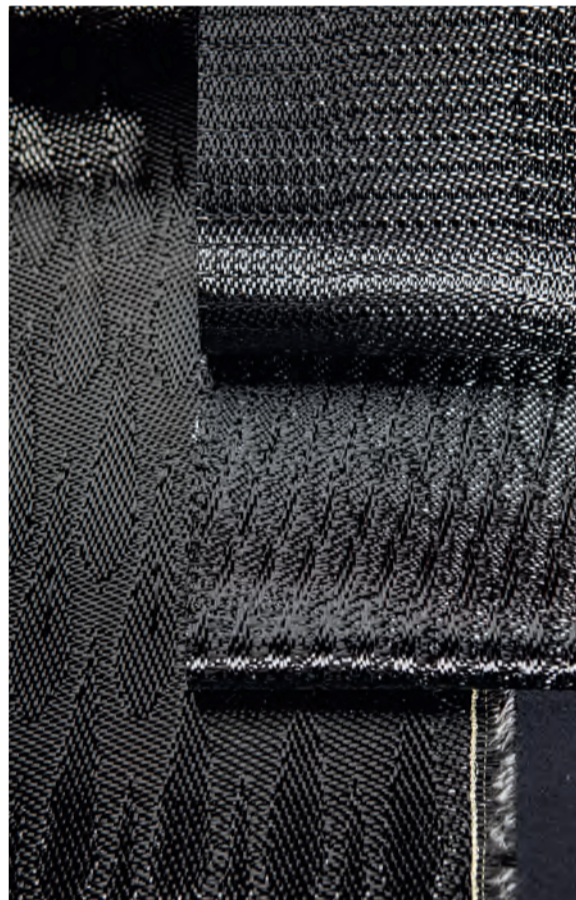
The Jacquard loomed carbon fibre reveals the patterns woven in according to the light
