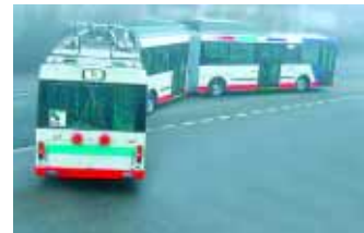
Vossloh Kiepe's double articulated trolleybus with four axles can accommodate up to 200 passengers. Known as the light tram, the vehicle is in use in Geneva.
