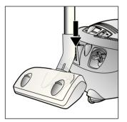
You can use the parking aid on the back of the appliance during short pauses in vacuuming after switching off the vacuum cleaner. To do this, slide the catch on the floor tool into the groove on the back of the appliance.
