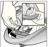
Open the cover by moving the locking lever in the direction of the arrow.
