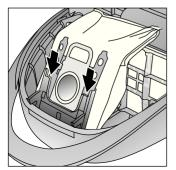
Place a new MEGAfilt\*SuperTEX dust bag in the holder and close the dust bag compartment lid.
