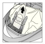
Seal and remove the  $\ensuremath{\mathsf{MEGAfilt}}^{\ensuremath{\mathsf{SuperTEX}}}$  dust bag by pulling on the tab as shown.
