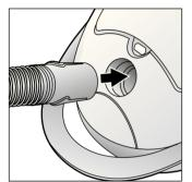
Insert the flexible hose connector into the opening on the vacuum cleaner until it engages.
