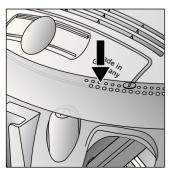
The button can also be pressed using the swing handle.
