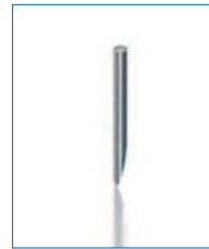
Stylus tip 33 mm Order no.: 101-010-330 made of carbide, \varnothing 3.5 mm / R: 25 \mu m / A: 12°
