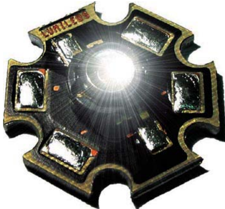
Fig. 2.28: High-current LEDs from LumiLeds mounted in a plastic lens filled with silica gel.
