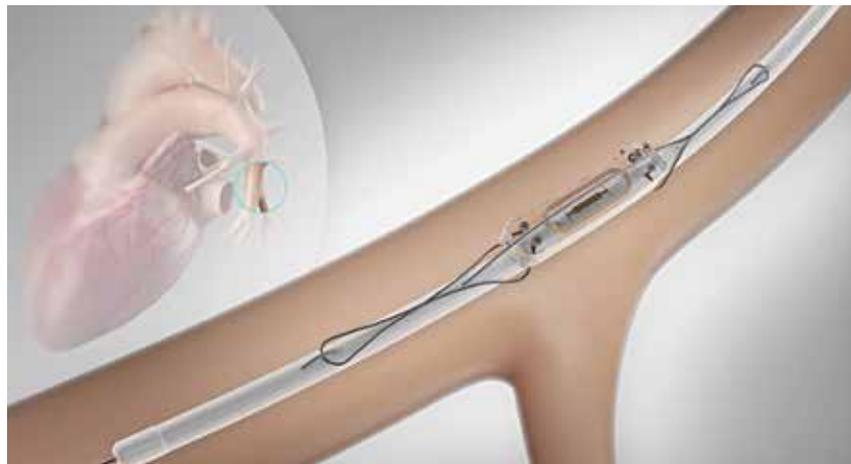
**Figure 1.** CardioMEMS heart failure monitoring system showing the target location for the pulmonary artery pressure sensor.
