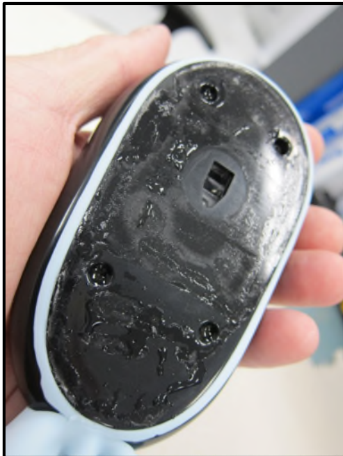
Figure 17: Water under adhesive label overlay
