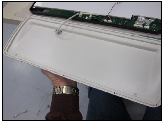
Figure 10: No evidence of ingress on the bottom housing
