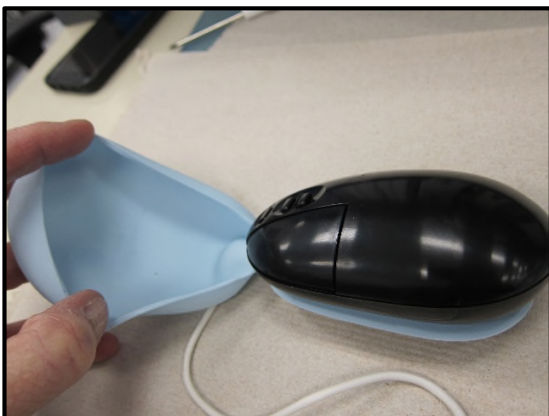
Figure 15: No water under elastomer
