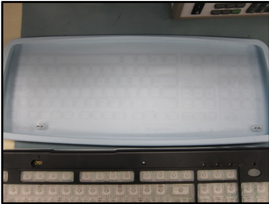
Figure 7: The underside of the elastomer overlay is dry.
