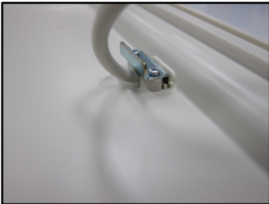
Figure 11: Cable exit was dry.
