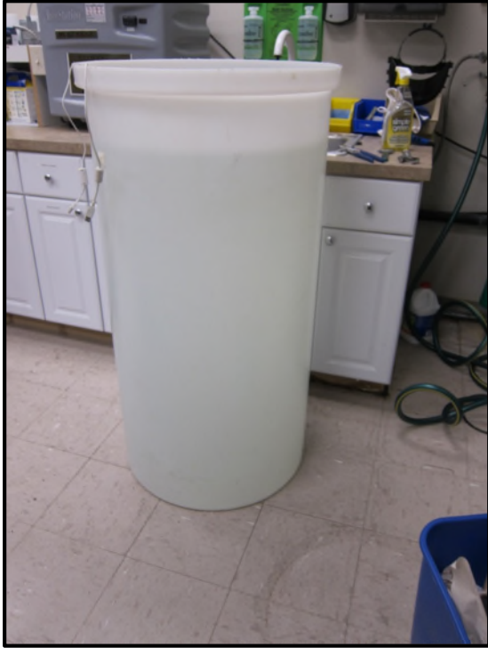
Figure 1: 1-meter deep dunk tank used for IPX7 testing.
