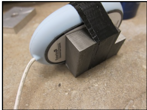
Figure 4: Metal sinker taped to mouse.
