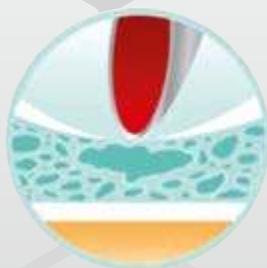
Figure 2: Under increasing pressure, the thin membranes tear, that separate the drops of the gel. A larger contiguous amount of anti-microbial, gel-like fluid is formed.
