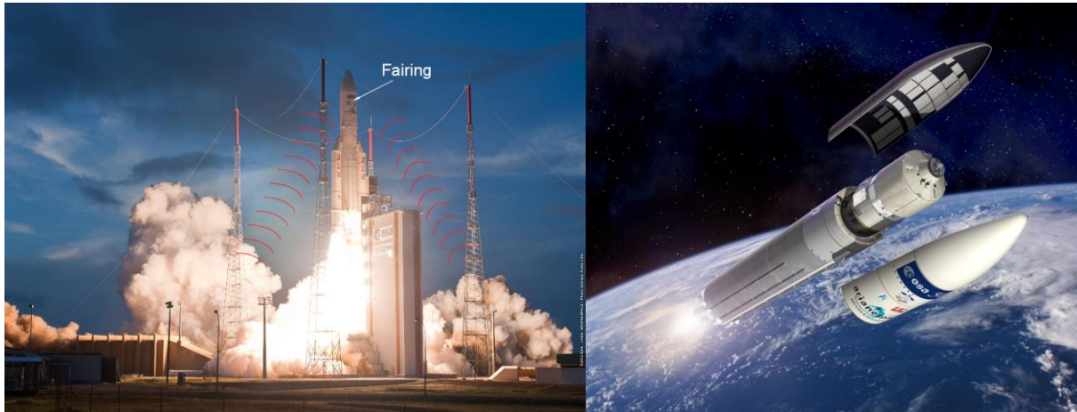
Figure 1. Left: Ariane 5 lift-off (Flight V209); right Fairing separation from Ariane 5 last stage when leaving earth atmosphere.
