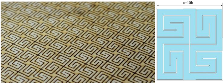
Fig1. Chiral lattice hinge plate and a unit cell with a rib/slit length ratio of 10
