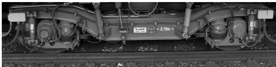
Figure 1. Renfe CIVIA bogie featuring primary rubber elements [4].
