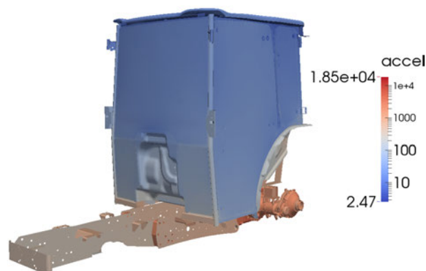
Figure 2: DEA results for the acceleration (given here in mm/s^2 ) at a frequency of 1000 Hz.
