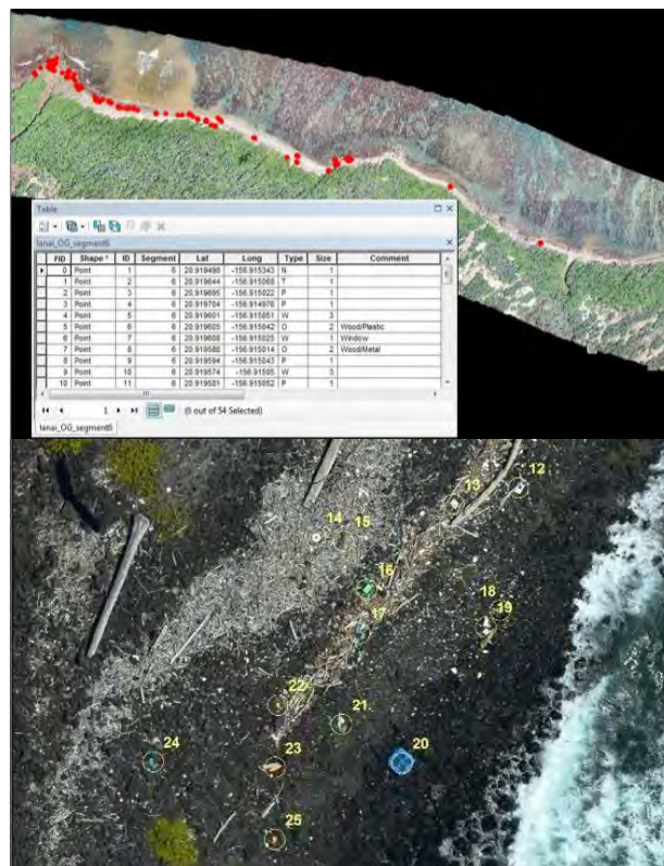
Figure 6-1. A swath of Kaua'i coastline in ArcGIS and the data table of the identified dots of debris (left), with a zoomed screenshot of identified marine debris with numbers on Kamilo Point, Hawaii Island (right).
