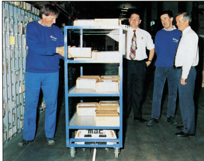
Lurking beneath the trolley which Keith Russell is loading with 'W' items is a 'little MAC' AGV which pushes the trolley along and takes it right into the adjoining assembly building. Trials commenced in July and the plan is to introduce a second AGV. Watching are (l. to r.) Paddy Weir, Sean O'Connell and Des Halliday.
