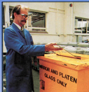
In the dismantle area in building 5, John Austin 'posts' a platen glass from a 1025 in one of the new containers. "We used to put mirror and platen glass in a skip along with other material - this way it doesn't get contaminated and can be recycled," says John.
