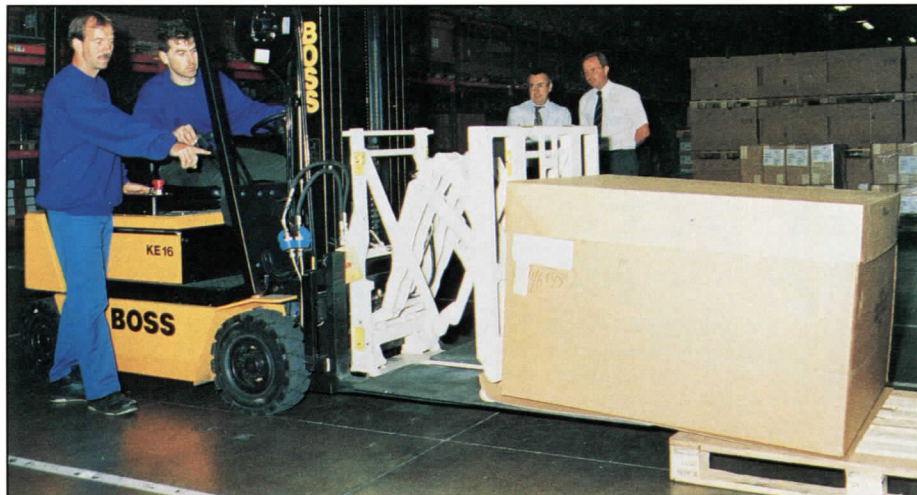
Roger Foxwell shows Jerry O'Connell how to operate the forklift specially adapted for pallet-less handling. The cardboard slipsheet with its load is drawn pneumatically off a recycled pallet (used for storage) and delivered to the line.
