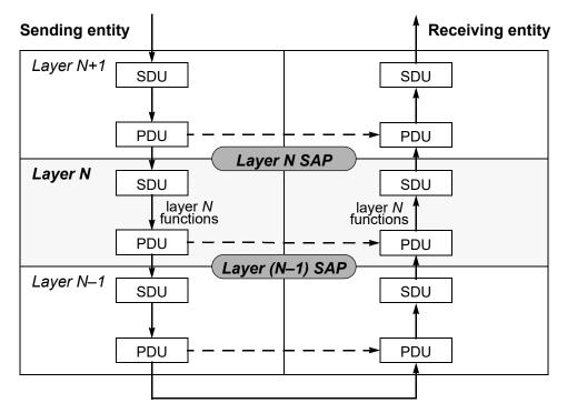
Figure 3-1—PDU and SDU in a protocol stack
