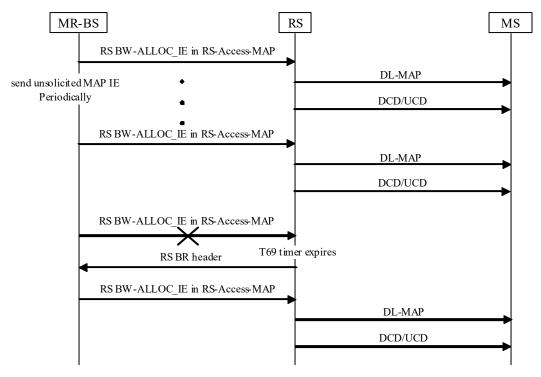
Figure 6-9—DCD/UCD broadcasting procedure with an RS operating in centralized scheduling mode
