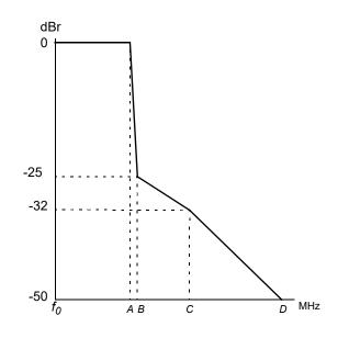
Figure 8-1—Tx spectral mask (see Table 8-2)
