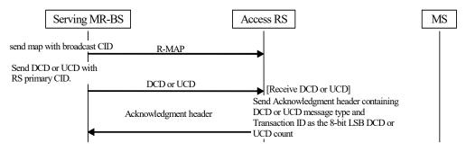
Figure 6-8—Relaying DCD/UCD procedure
