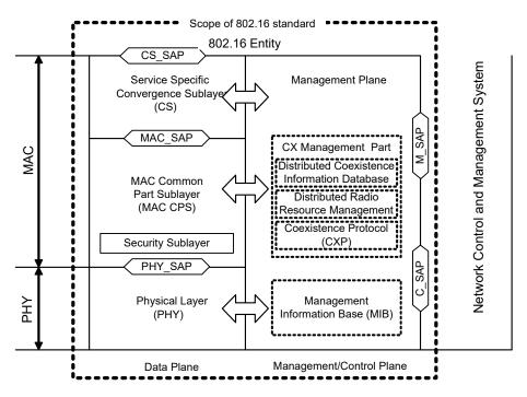
Figure 1-1—IEEE 802.16 protocol layering, showing SAPs
