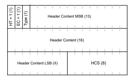
Figure 6-6—MAC signaling header type II format
