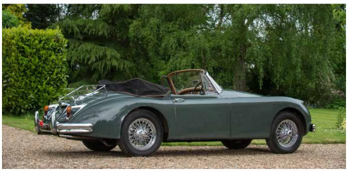
Overdrive and a Borg-Warner automatic gearbox were the transmission options, the latter becoming an increasingly popular choice, while a Thornton Powr-Lok limited-slip differential was available for the XK150S. Steel wheels remained the standard fitting, though XK150s so equipped are a great rarity, as most were sold in SE (Special Equipment) specification with centre-lock wire wheels. The much admired chromed Jaquar mascot was made available as an optional extra on an XK for the first time.
