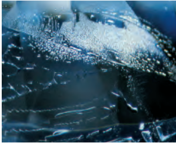
Figure 26. Two-phase inclusions are not commonly seen in benitoite. The larger inclusions in the healed fracture of this 0.95 ct stone contain vapor bubbles of variable shape and size. Darkfield illumination, magnified 25 \times ; photomicrograph by John I. Koivula.
