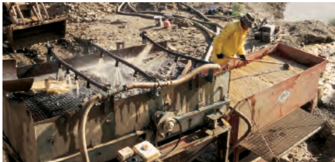
Figure 17. At the Benitoite Gem mine, material is fed first into a layered screening apparatus fitted with high-pressure water jets, and then into a gravitational separation jig. Pieces over 25 mm are separated by the screening apparatus and checked for specimen potential, while material between 3 and 25 mm is washed into the jig where the heavier benitoite is trapped in several parallel trays. Photo by Brendan M. Laurs.
