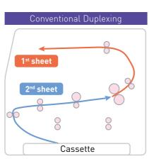
After printing both sides of 1<sup>st</sup> sheet, printing of 2<sup>nd</sup> sheet starts.
