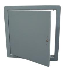
The MIFAB EA is a multi-purpose access door. It is designed for flush installation into drywall, block or tile walls and ceilings. Frame features rounded safety corners, concealed hinge, flush with frame fit, and a 3/8" turn back in the door panel for extra rigidity and safety.
